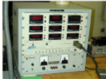
011105 Generator test bench.JPG
